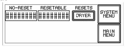
This screen monitors the number of hours that the dryer, machine blower, and dryer blower have operated.
